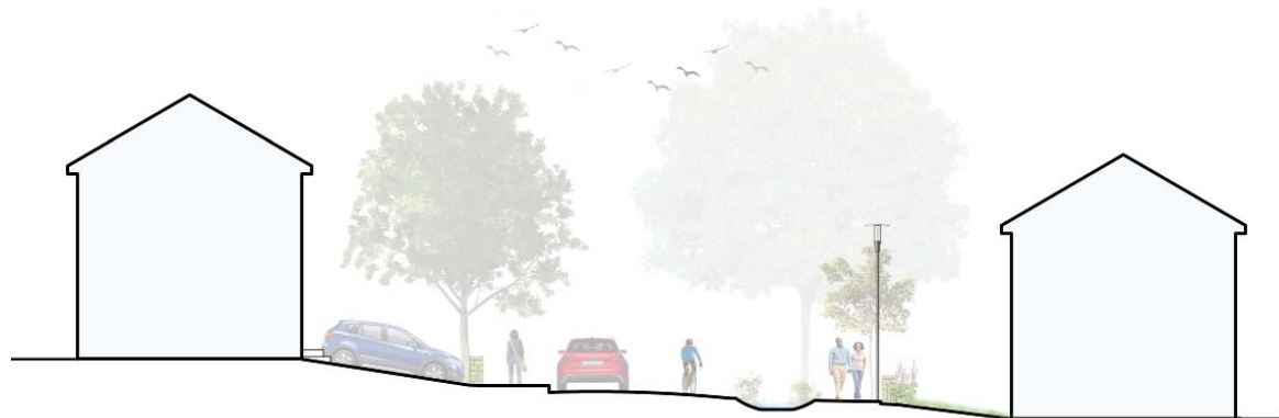
Street section showing an example of a connecting street in the framework plan which incorporates sustainable drainage through the use of swales
